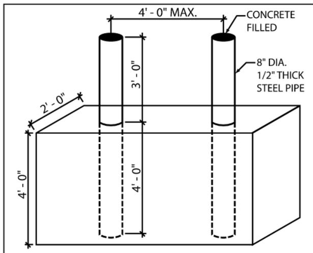
Fig 3: Steel bollards used as Barriers for 4500 lbs. vehicle travelling at 30mph<sup>5</sup>.
