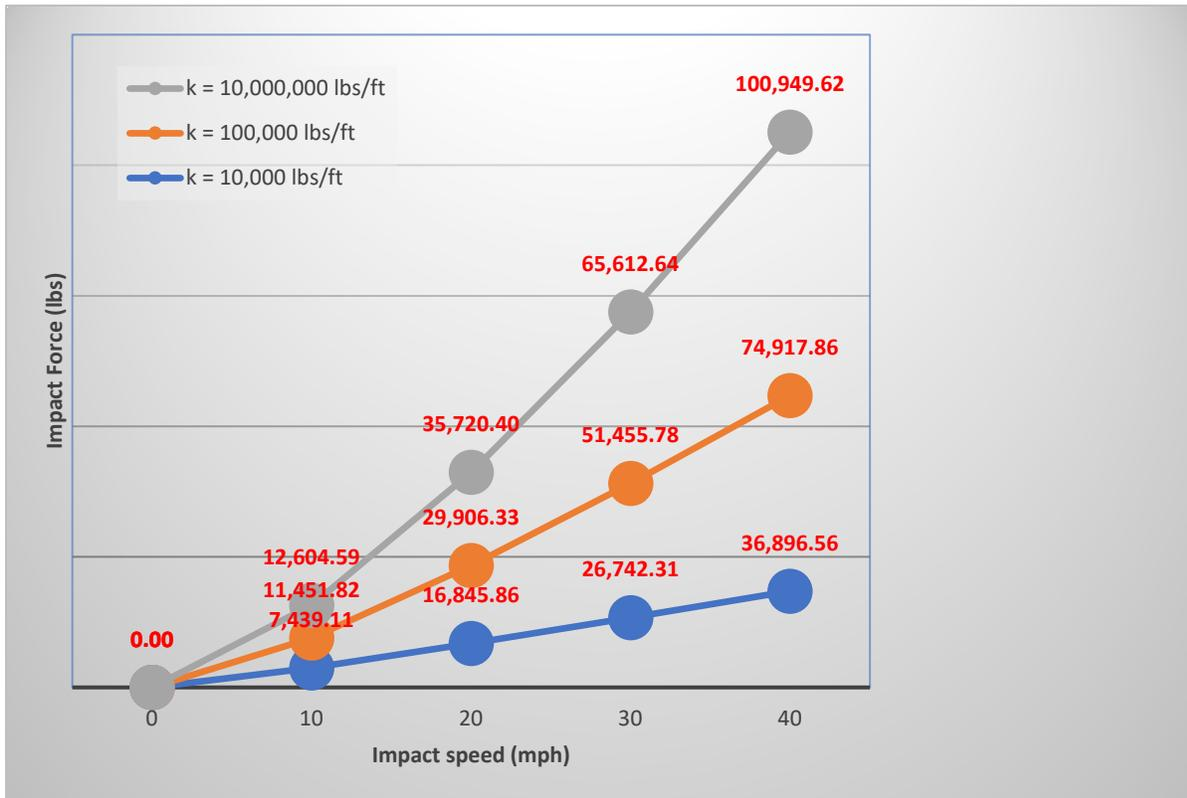
Fig 4: Vehicular Speed-Impact force plot for a 4000 lbs. vehicle with barrier stiffness, k.(NTS)
