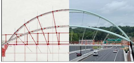
**A.** In the same way that an Excel spreadsheet updates on input changes, parametric design updates 3D geometry and the supporting engineering analyses, live and in real time. It's as simple as watching the span of a bridge change in front of your eyes by changing the end point coordinates, yet extremely powerful because of the computational design automation that is connected to those points which automatically updates as the spatial relationships are changed or defined.
